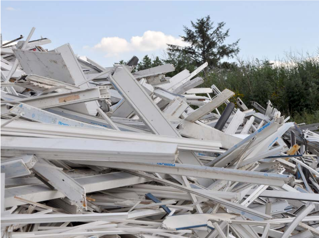
Window profiles ready for mechanical recycling. With a market share of almost 40 %, PVC is the most used plastic material in building and construction. Window profiles, pipes, doors, cables, flooring, roofing membranes and other long-lasting applications are often made of PVC. These are easy to collect and recycle into new products.
